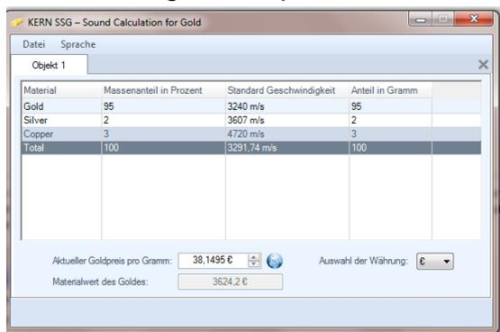
This calculated ultrasonic speed must now be entered into the SAUTER TN-US ultrasonic measuring device.
