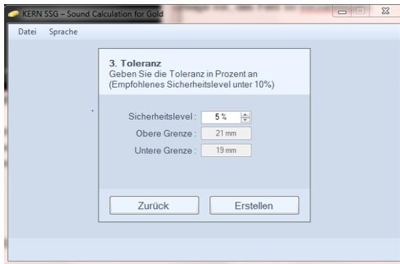
If the measurement result is above or below the tolerance range, it is recommended that a comparative measurement be made at another point on the gold piece, or on the other two opposite side faces (for bars).
