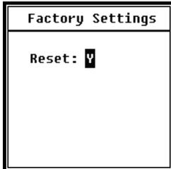
**Factory settings** offer the possibility to reset all parameters that have been changed by the users to the factory settings. The parameters are initialized with the default values. Use the arrow keys <◀>, <▶> to select Y (Yes) or N (No). If you select Y (Yes) and **press** the <Enter> key, the parameter will be initialized. If you select N (No) or press the **ESC key**, the reset will be cancelled.
