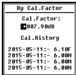
Select the **With calibration factor** option and press the <Enter> button to enter the menu.
