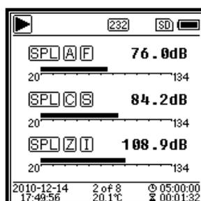
Main screen Displays measurement data, filter, detector, mode and profile number. The main screen shows only one data group of the 3 profiles. Press the arrow keys **<▲>** , **<▼>** to switch **between** the 3 profiles.
