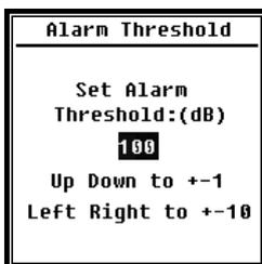
If measurement results of profile 1 - 3 exceed the **alarm threshold**, the LED above <Power> will light **red**. The alarm threshold can be set between 20 dB and 200 dB. Use the arrow keys <▲>, <▼> to increase or decrease the alarm threshold by 1 dB. Use the arrow keys <◀>, <▶> to increase or decrease the setting by 10 dB.
