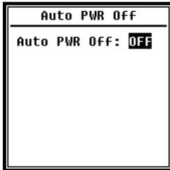
The sound level meter has an automatic switch-off function to reduce power consumption. If the sound level meter remains in stop status and no button is pressed for a certain period of time, the instrument will shut down according to this setting. The following settings are available for the auto power off option: **1 minute, 5 minutes, 10 minutes, 30 minutes, Off**. Press the arrow keys < ◀ ▶ > , < ▶ ▶ > to select. Press < Enter > to save the setting.
