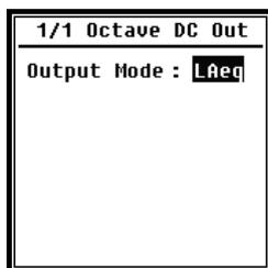
**1/1 Octave DC Out** defines the output signal in 1/1 octave mode. The following options are available: LAeq, LBeq, LCeq, LZeq, 31.5 Hz, 63 Hz, 125 Hz, 250 Hz, 500 Hz, 1 kHz, 2 kHz, 4 kHz, 8 kHz, 16 kHz. Press the arrow keys <◀> , <▶> to select.
