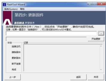
**Step 4:** First press the button in the upper right corner to select the firmware and then press the **Update** button to start the program. The whole procedure takes 3 to 4 minutes.
