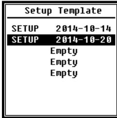
The setup template allows you to save five user group setting parameters of the sound level meter for different applications.
