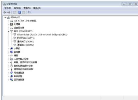
After installing the driver, connect the sound level meter to the computer with a USB cable. In the Device Manager, you will find a new device called **Silicon Labs CP210x USB to UART Bridge (COMx)**.
