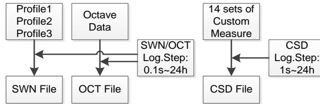
☆ **Note:** A SWN/OCT file can only store integral data. The logging step can be considered as an integral period. All data within the logging step (the integral period) is saved as one line in the SWN/OCT file. The CSD file only saves instantaneous data without integration. As soon as the CSD logging step is reached, the 14 group data of the adjustable measurement are saved as a line in the CSD file like a snapshot.
