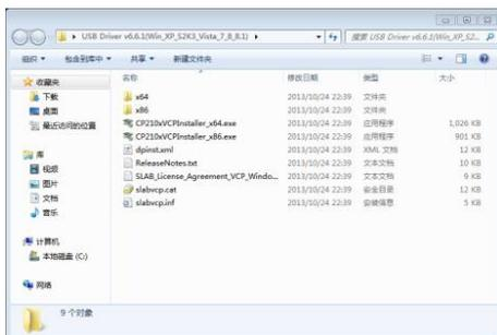
Unpack and install the driver step by step. Select X86 for a 32-bit operating system and X64 for a 64-bit operating system.
