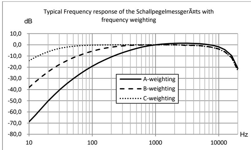
The following table shows the influence of the upper limit of the measuring range with A, B and C weighting and a typical frequency response as shown in the figure:
