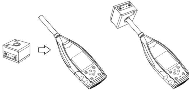
2. Then switch on the calibrator and set a constant sound level (for example 94 dB).
