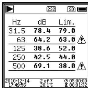
Octave table page 1. display of measured data from 31.5 Hz - 500 Hz. The LED lights red and ⚠ appears when the data exceeds the threshold value.
