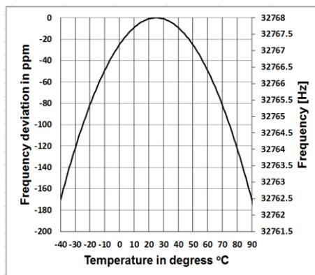
The accuracy of the system clock may vary depending on the temperature, as there is no temperature compensation. With the typical temperature curve in the illustration, the system clock does not change its base frequency. If the temperature rises or falls, the frequency of the system clock changes by about  $-0.04 \text{ ppm}/^\circ \text{C}^2$ . Therefore, if the temperature is  $0^\circ \text{C}$ , the value for the system clock changes by  $-0.04 \times (0-25)^2 = -25$
