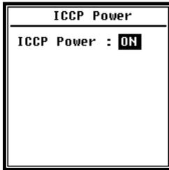
The ICCP menu controls the power supply of all ICCP sensors via the 24 V/4 mA constant current source. Disable the ICCP power supply before connecting another sensor or connecting directly to the signal source. Press the arrow keys <◀>, <▶> to select.
