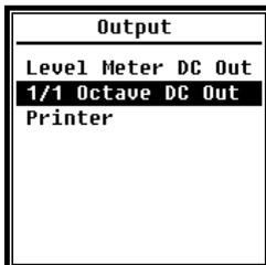
For the **Output** menu, you can select which measurement data are to be output at the **DC voltage output**. For **Level Meter Mode** and **1/1-octave mode**, there are Level Meter DC Output and 1/1-octave DC Output options.
