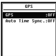
In the **GPS** menu you can enable or disable the **GPS** and **Auto Time Sync** options. When the **GPS** is disabled, the internal GPS module is turned off. The system clock of the sound level meter will synchronize with GPS time if you enable the **Auto Time Sync** option.
