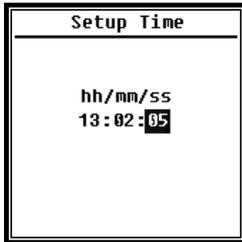
Changing the time setting is similar. Use the arrow keys <◀> , <▶> **to** select hour, minute and second and use the arrow keys <▲> , <▼> to modify the value. Press <Enter> **to save the setting.**
