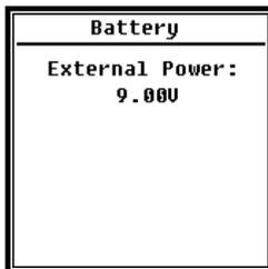
The **Battery** menu displays the battery status and voltage.
