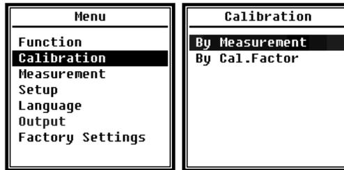
4. Set the value for **Cal.Level** in the menu, for example to 93.8 dB. Calibration is performed 5 seconds after pressing the <Start> button.
