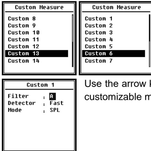
There are 14 **adjustable measurement** menu options where you can define the parameters for 1 - 14 adjustable measurements. Use the arrow keys <▲> , <▼> to select the option and press <Enter> to move to **the next menu level**.
