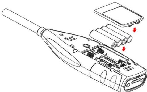
Replace the batteries and close and lock the battery compartment.
