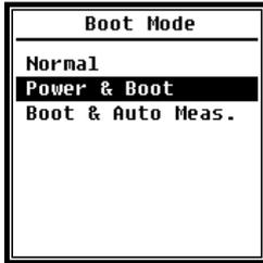
In **Start mode**, use the arrow keys <▲>, <▼> to select **Normal**, **Power & Boot**, and **Boot & Auto Meas.** (Switch on and Auto Meas.).
