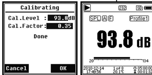
6. Go back to the **main screen** and press <Start/Stop> to start the measurement. The current measurement result in this example is 93.8 dB if the calibrator is in good working order.
