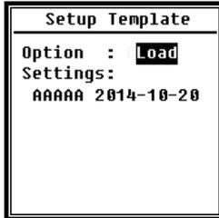
Press the <Enter> button **when the** template is empty. The template can store a group setting for which the user can specify a five-letter or numbered label.
