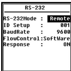
The RS-232 interface menu is used to set the options for the serial connection, see 5. [RS-232 data exchange protocol](#).
