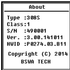
The About menu displays the type, class and serial number, version and HWID (hardware ID) of the sound level meter.
