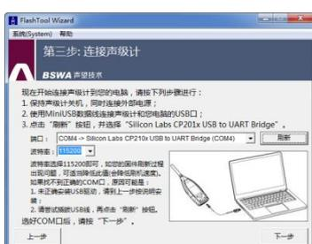
**Step 3: Connect** the sound level meter and the computer according to the user's request. Note that the sound level meter requires an external power supply. If the driver is working properly, it will automatically select the CP210x **connector**. The default value for **baud rate** is 115200 bps, depending on the computer. With a higher **baud rate** the update procedure can be accelerated.
