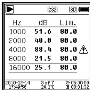
Octave table page 2. display of measured data from 1 kHz - 16 kHz. The LED lights red and ⚠ appears when the data exceeds the threshold value.
