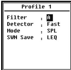
The menu for the profiles 1 - 3 allows the definition of the filter, the detector, the mode and the storage options of SWN files. Options can be selected with the arrow keys <▲>, <▼>.
