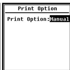
The **Print** option allows you to set the printer to print automatically or manually. If you select the **Auto** option, measurement results are printed automatically after the measurement stops.
