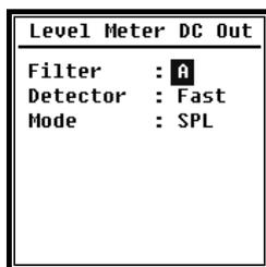
The **DC output** of the level meter can set the signal output for the level meter mode. Press the arrow keys <▲> , <▼> , <◀> , <▶> to select.
