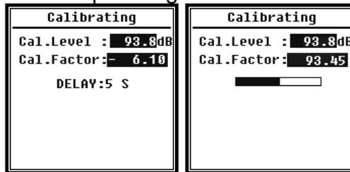
5. When the calibration is finished, the sound pressure meter updates the calibration factor. Press the <Enter> button to accept the results.
