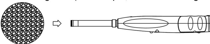
Press the windscreen firmly onto the microphone as shown in the figure above until it stops. See [Appendix 4 for](#) more details on how to adjust the windshield outdoors.
