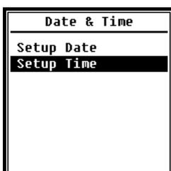
In the **Date & Time** menu the RTC time of the sound pressure meter can be set. Press the arrow keys <▲>, <▼> to select.
