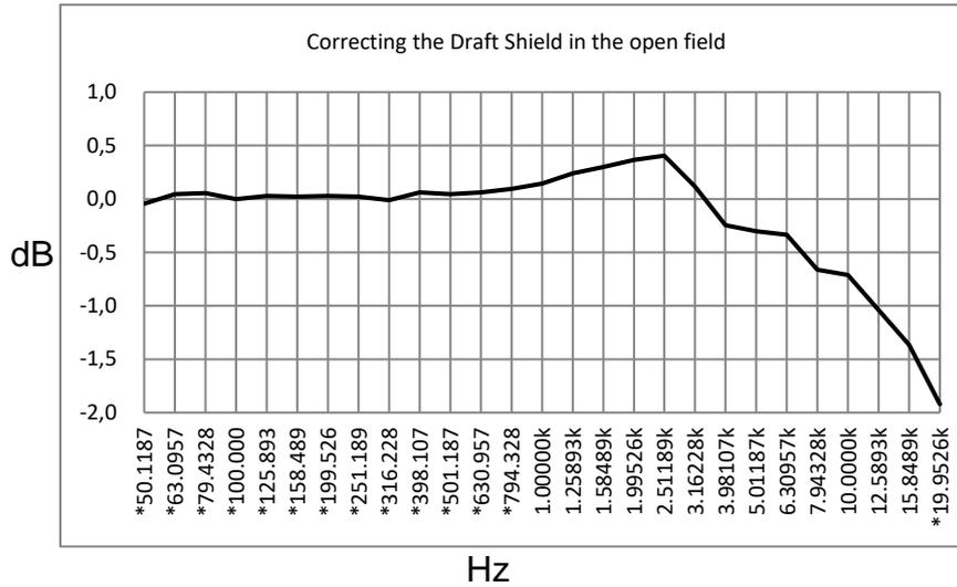
Note: The frequency marked with \* is not prescribed in the standard, the exact frequency can be found in IEC 61672-1.
