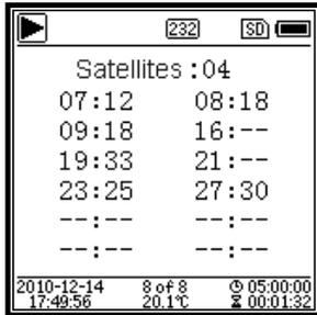
GPS page 2. display the number of satellites for positioning and the signal-to-noise ratio of all visible satellites (0 dB - 99 dB).
