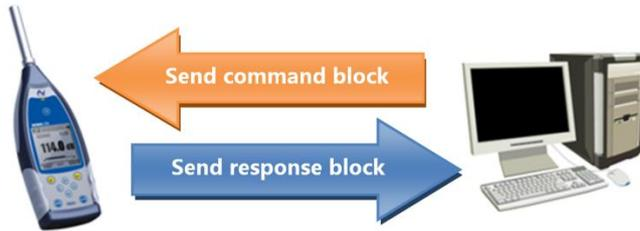
A typical command block or response block consists of a start character, the ID, the attribute character, the command or data, the end character, the block check character, the carriage return and carriage return characters, as shown in the following figure:
