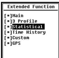
With the advanced function, you can set which screen is displayed. If the screen is not selected, it is not displayed. Note that the **Main Menu** screen is always displayed.
