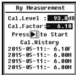
Select the **By Measure** option and press the <Enter> button to enter this menu. See Chapter 7 for more details on the specified calibrator and its corresponding adjustment values.
