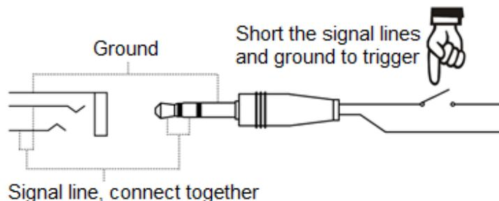
The measurement is started by connecting the signal line to ground and stopped by interrupting it. Note that when the **trigger function is** activated, the <Start/Stop> **button** is not available.
