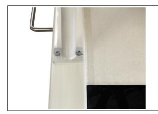
Carefully mount the rail and fasten it with screws.
