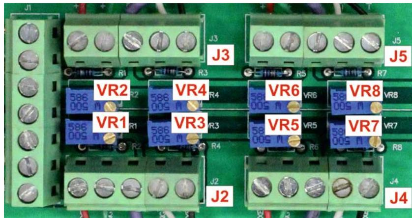
Adjustment of weighing cell J2 takes place at the potentiometer VR1 and VR2.
