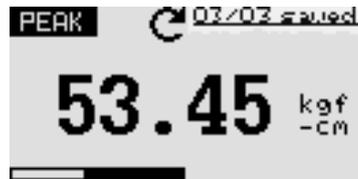
Press the arrow keys UP or DOWN to change the memory mask. Press and hold the key to scroll to the position for changing the memory mask. Pressing the PRINT key controls the print output of stored data and data transmitted via serial port. To access the *DELETE* menu screen, press the ZERO key.
