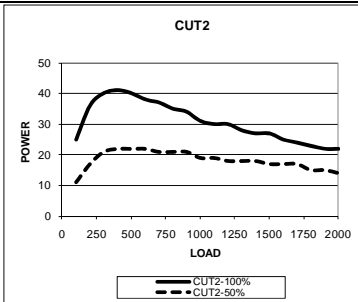
Diagrams of half and maximum output power versus impedance load 100-2000Ω CUT2
